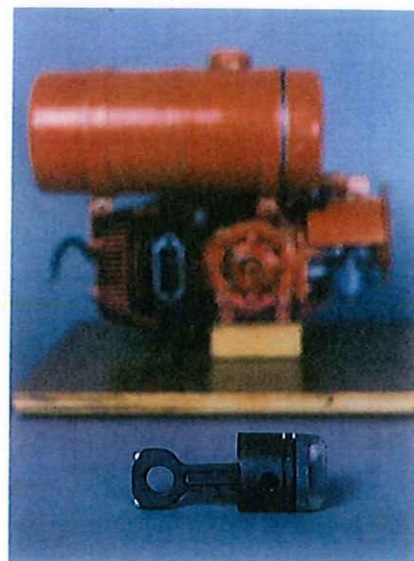
At Western Michigan University, a 5 hp engine with TORLON power train components has run successfully for more than 700 hours on the dynamometer.
