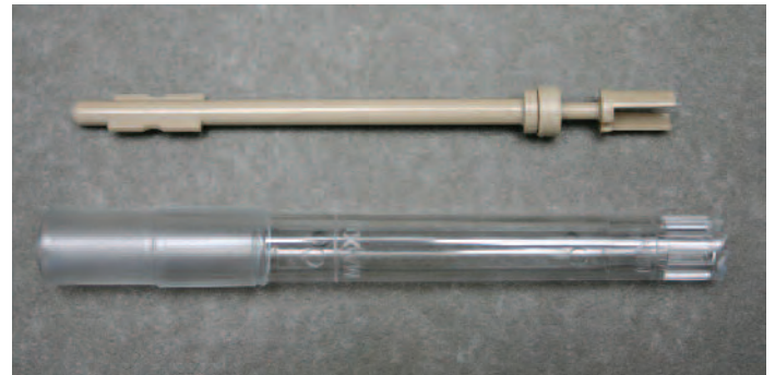
VICTREX ® PEEK polymer replaced steel in high-speed rotors and intricate bearing shells for dispersion instruments used in the medical industry.
