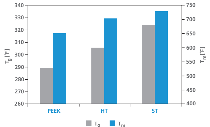
Figure 13: The glass transition ( T_g ) and crystalline melting temperatures ( T_m ) for Victrex polymers determined by differential scanning calorimetry (DSC) ISO 11357
